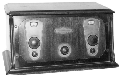
FREED-EISEMANN MODEL 30 – The Freed-Eisemann Corporation of New York manufactured this 6-tube battery set in 1926. It operates with the Neurodyne circuit using two tuning dials. (Clark Trissell – Lincoln, NB)
