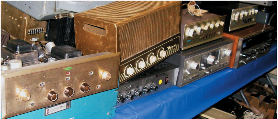
Offerings of early hi-fi gear included several items. Among them at left is an H.H. Scott Model 99C monorail amplifier, which includes a record compensation selector switch; it sold for $75. The large item, center, is a Masco ME27 amplifier, which sold for $155.
