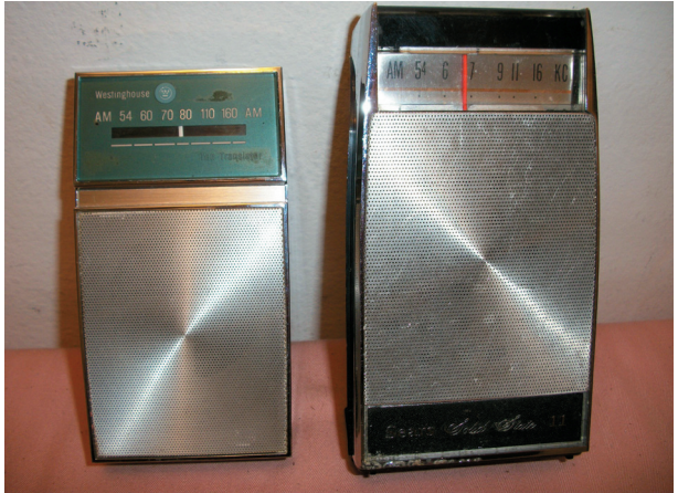
Left is the 10-transistor Westinghouse RG21S570, and right is the 11-transistor Sears 8212.
