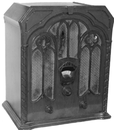
MAJESTIC MODEL 311 – Built in 1932 by the Grigsby-Grunow Co., this tombstone table radio uses the following seven tubes: (1) Type 80 rectifier, (1) Type 47, (1) Type 55, (1) Type 56, and (3) Type 58. (Clark Trissell – Lincoln, NE)
